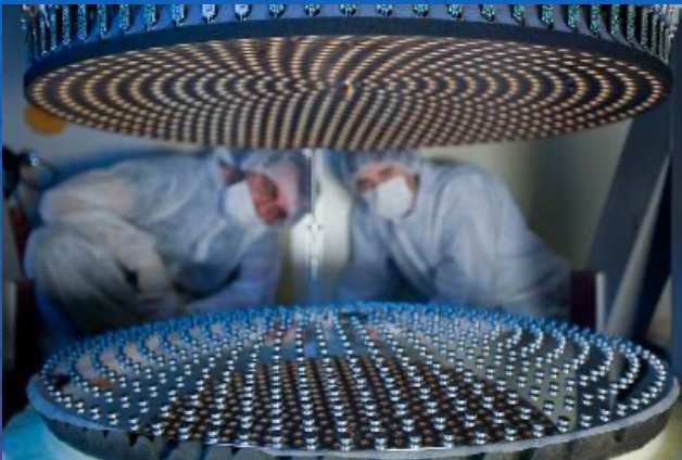
Large Binocular Telescope ASM showing facesheet with magnets
