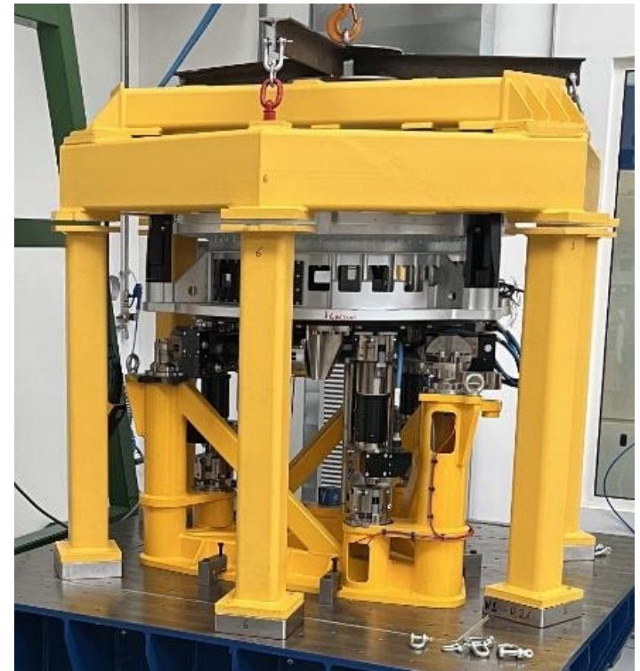
Testbed structure assembled with ASM simulator during Dry run of the integration procedure
