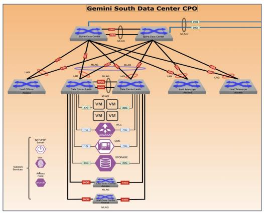
Example 2: Draft of CPO Network Design using L2 Spine-Leaf with Multi-Link Aggregation
