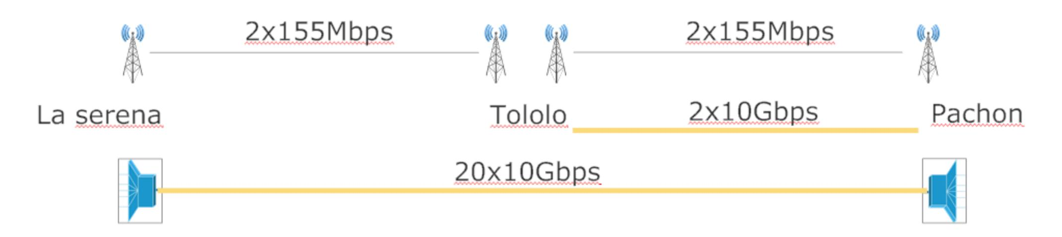
On 2018 new technology was install to give services to Vera —— Primary link Fiber Rubin and the rest of tenants, DWDM equipments. ——Backup Microwaves
