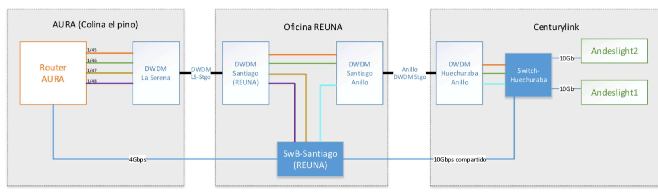
2 links from La Serena to Santiago. Primary is a 4 x 10Gbps using a fiber through the interior valleys and the backup 4 Gbps using the cost.
