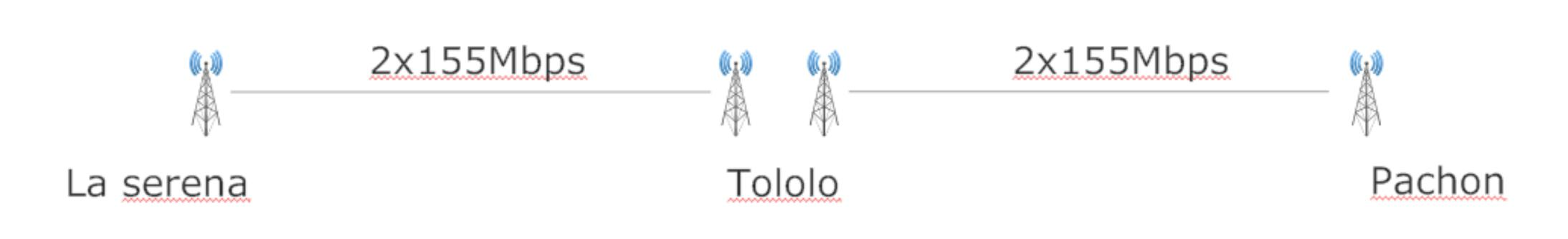
On the last century ->1985-1992 NASA provide a 64Kbps link On 2000 GEMINI joint us providing 2 x 155Mbps link - Harris microwaves
